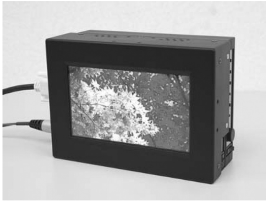
Figure 23. The prototype of 6.5-inch Full-HD field sequential color OCB-mode LCD.
